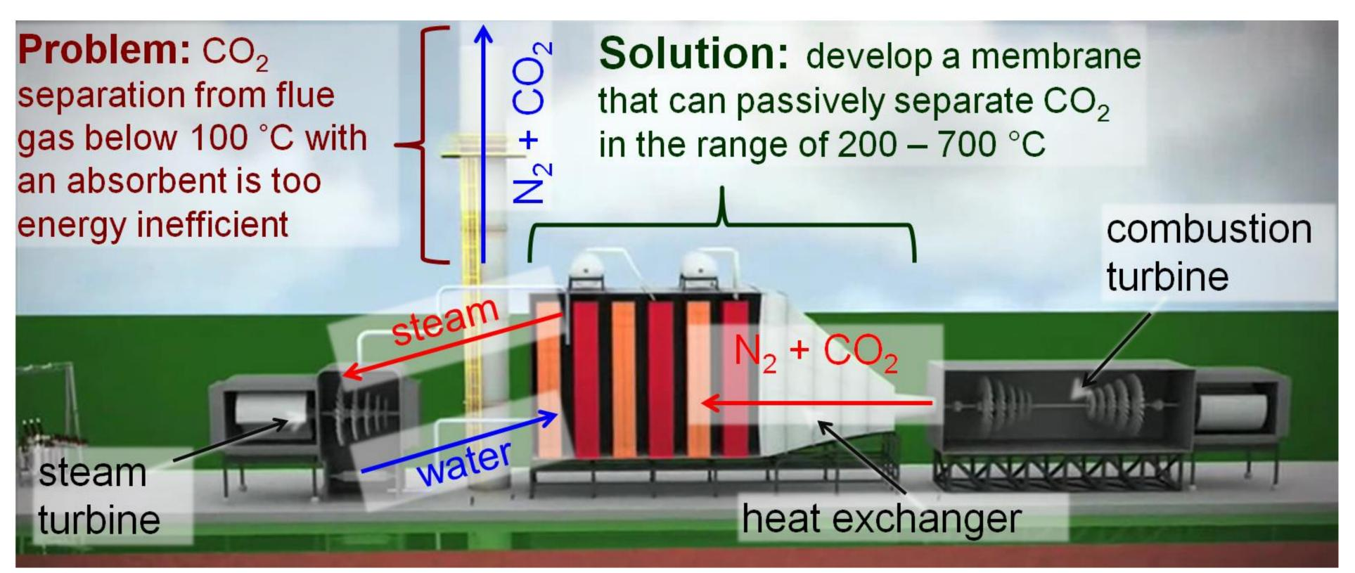
The dual phase membrane enables passive CO<sub>2</sub> separation from incipient flue gas in the temperature range of 200 – 700 °C and 1 – 20 ATM.
