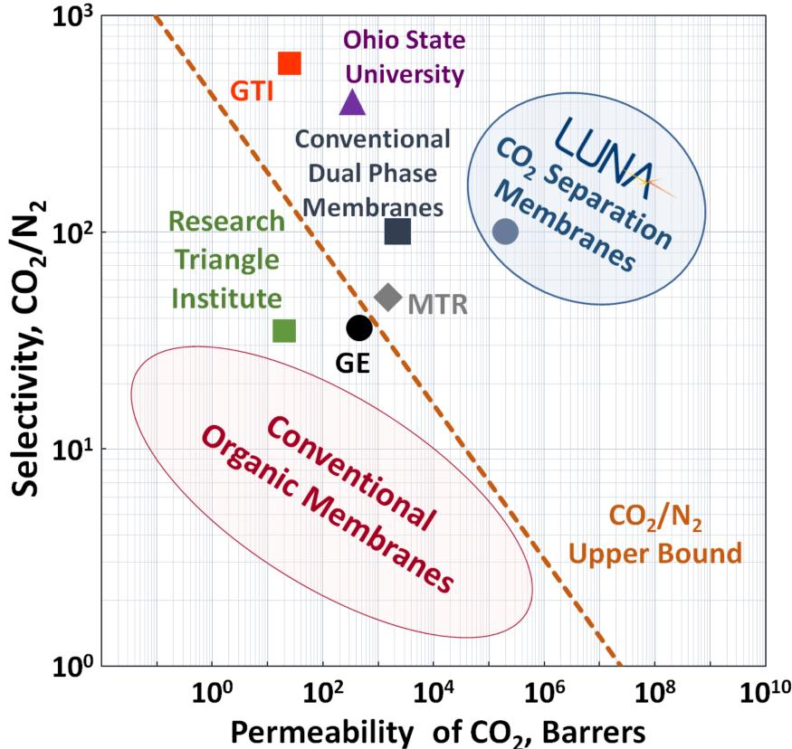
The dual phase membrane is similar to membranes used in molten fuel cells and is not limited by the physics governing Robeson's Upper Bound.
