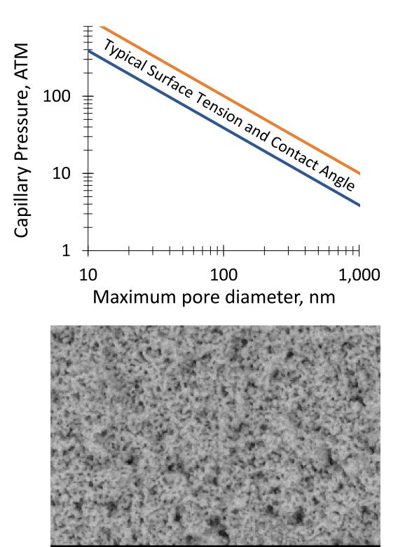
nanoporous, ceramic solid The phase retains the liquid separation phase with capillary action capable of withstanding 10's of ATM pressure gradients.
